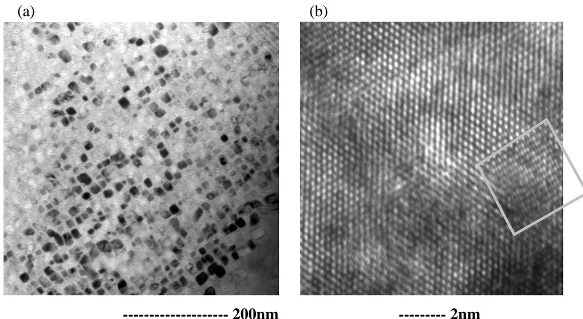
Figure 7. TEM of phase transformation,  $\beta \rightarrow \omega$ , in high strength pressure tube alloy EXCEL: (a) cuboidal hexagonal  $\omega$  particles in a matrix of body centred cubic  $\beta$ -Zr, and, (b) lattice image showing the atomic arrangement of both phases with a resolution of  $\sim 0.1\text{nm}$  ( $\omega$ -phase in the lower right quadrant marked by grey square). From the Ph.D. thesis project of Hongbing Yu.
