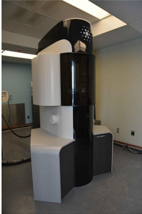
Figure 3. FEI Tecnai Osiris 200kV scanning transmission electron microscope at RMTL.
