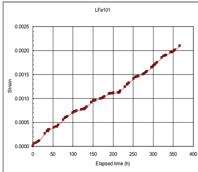
Figure 6. The same creep curve as Figure 5, but strain vs time, from Reference 4. The slope increases and decreases with increased and decreased beam current (proportional to displacement damage rate).
