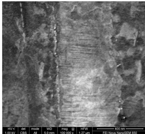
Figure 8. SEM image of what is probably a hydride in Zr-2.5Nb pressure tube material. The individual horizontal platelets of the hydrides ~15 nm wide are resolved.
