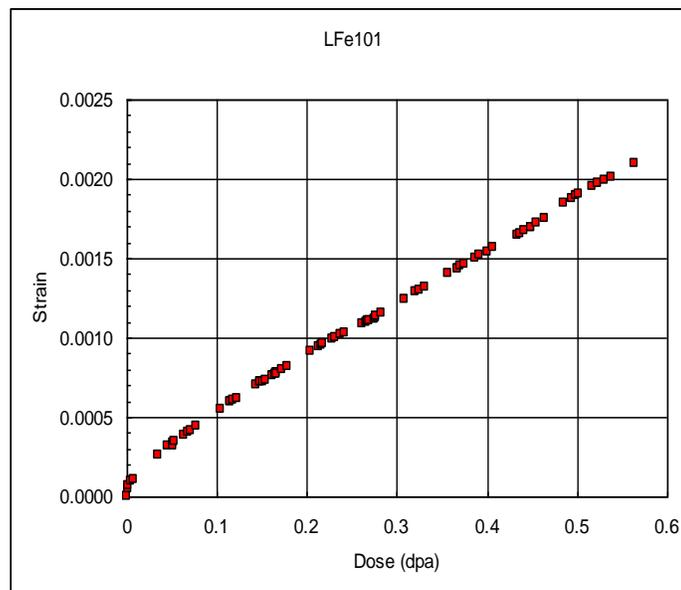
Figure 5. Creep curve (strain vs irradiation dose) for Zr containing 60 ppm Fe, irradiated with 4.4 MeV protons at 347 K with a stress of 50 MPa and various beam currents, from Reference 4.
