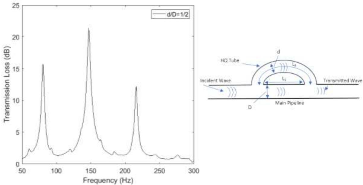
Figure 3: Effect of Herschel-Quincke placement along the piping system on the acoustic transmission loss
