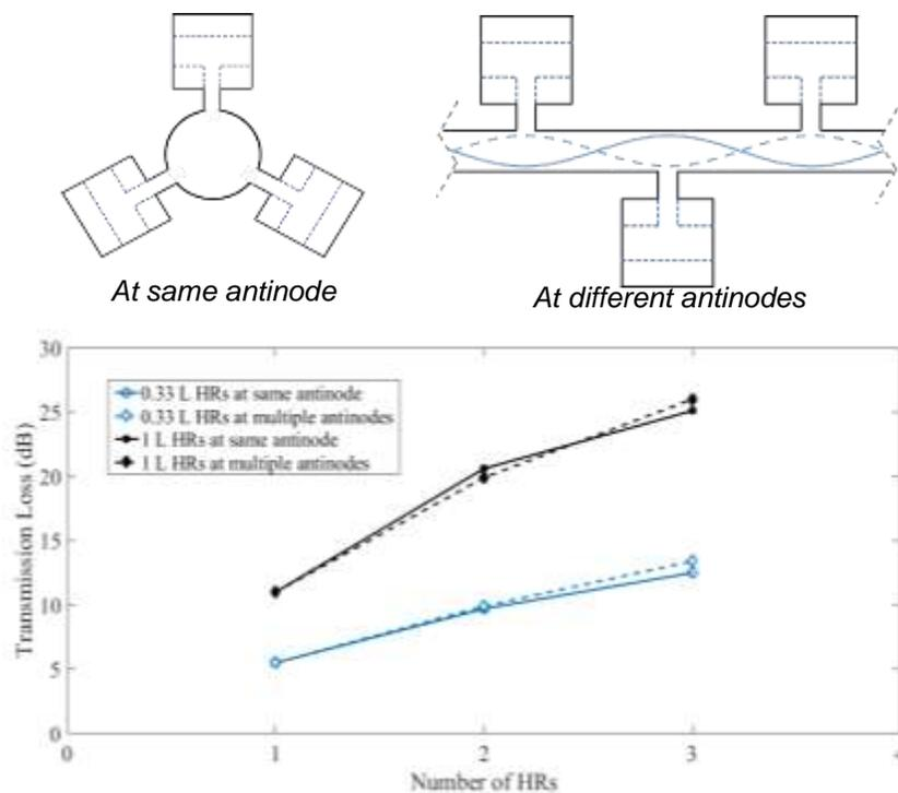
Figure 2: Effect of HR volume and location along the piping system on the transmission loss
