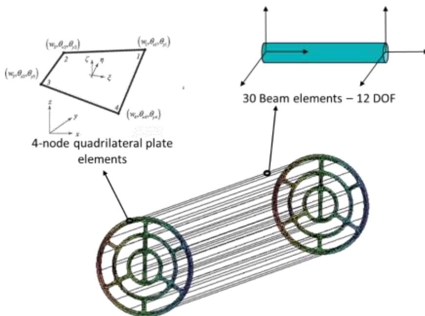
model represents the fuel rods by 30 beam elements each of which has 12 degrees of freedom. In addition the endplates is discretized by 1222 plate elements. A four-node isoparametric quadrilateral element was used to model both endplates. The 37 rods were coupled with the two endplates by utilizing common 74 nodes between the beam element and plate element.
