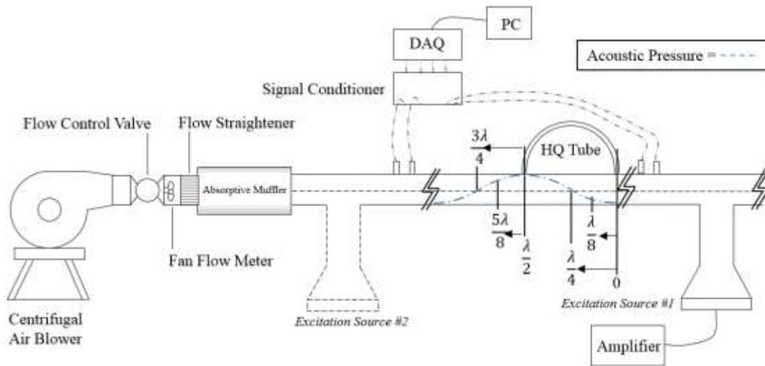
Figure 1 - Schematic of the experimental set-up for the air loop pipeline system
