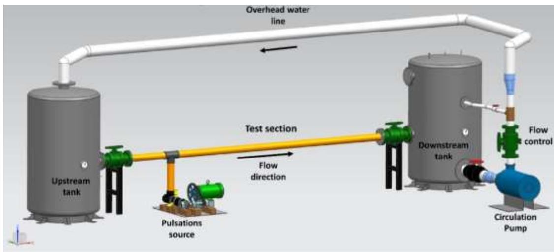
Figure 6: 3D CAD of the water loop that was commissioned for this project
