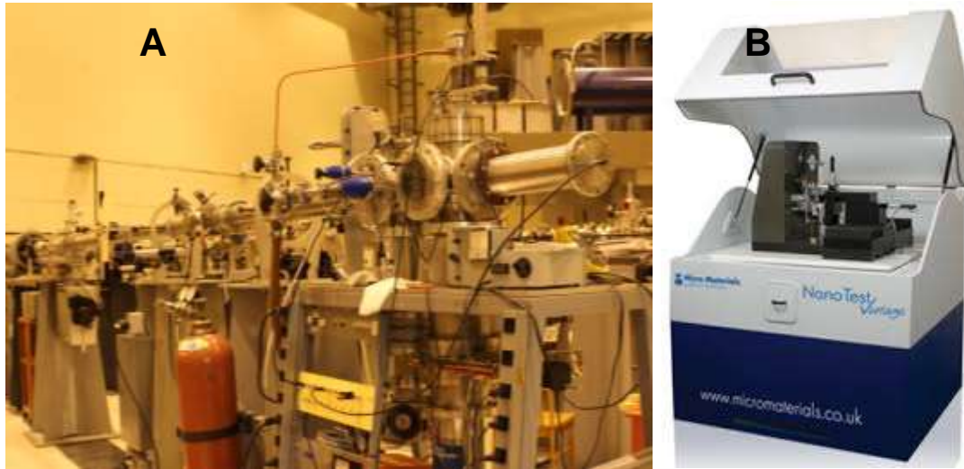
Fig. 1 A) An accelerator @ University of Montreal was used for irradiation and helium implantation of samples. B) A Nano-Indentation @ Queen's University was used for mechanical testing.
