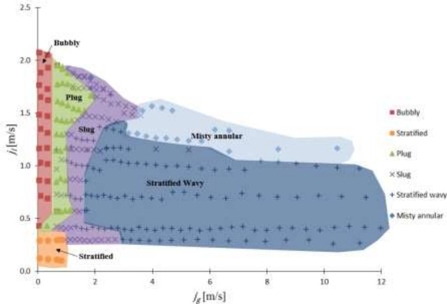
Figure 2: Flow regime map for horizontal air-water pipe flow study.
