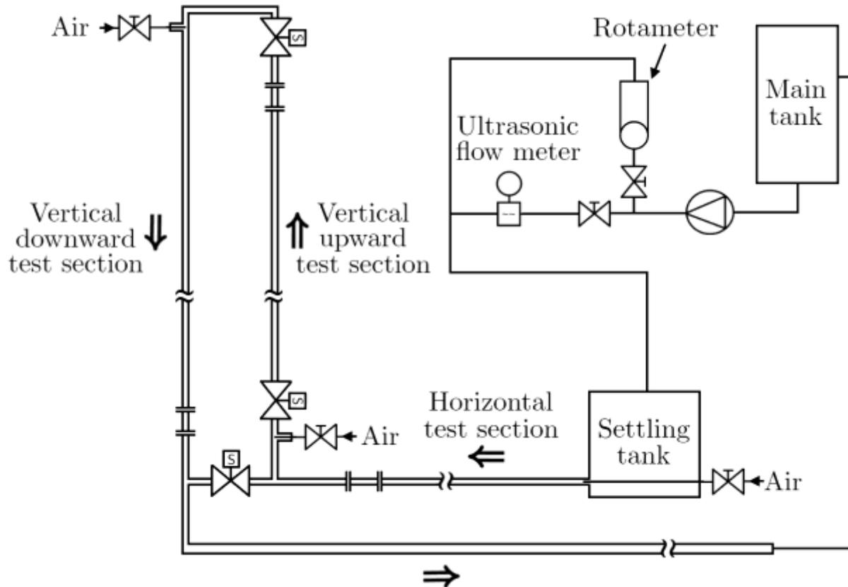
Figure 1: Schematic diagram of the water-air flow loop.
