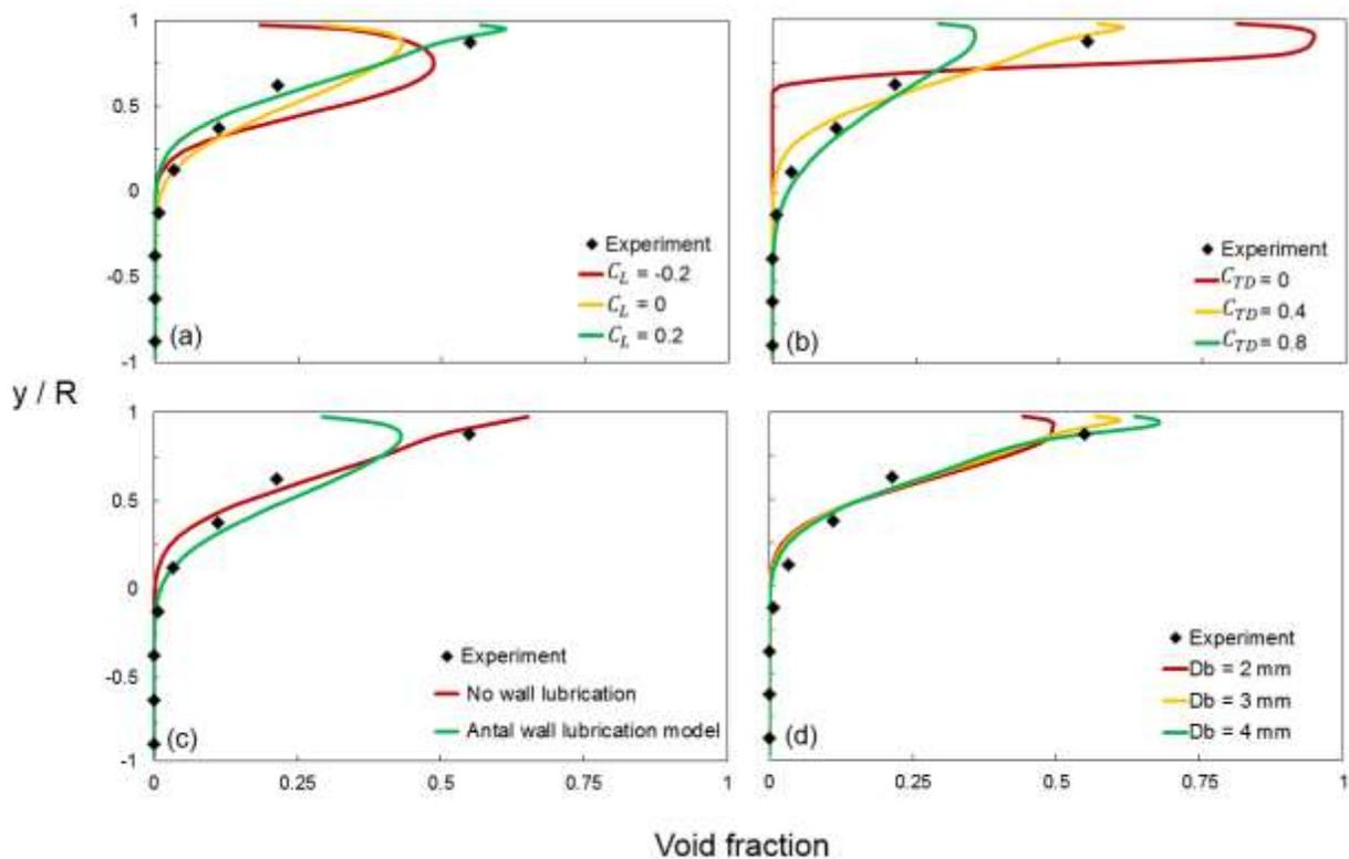
Figure 5: Effect of various model parameters on the radial void fraction distribution in horizontal air-water flow ( $j_L = 1.66$  m/s,  $j_G = 0.15$  m/s); (a) effect of the lift force coefficient, (b) effect of the Bertodano turbulent dispersion coefficient, (c) effect of the Antal wall lubrication force and (d) effect of the bubble diameter.
