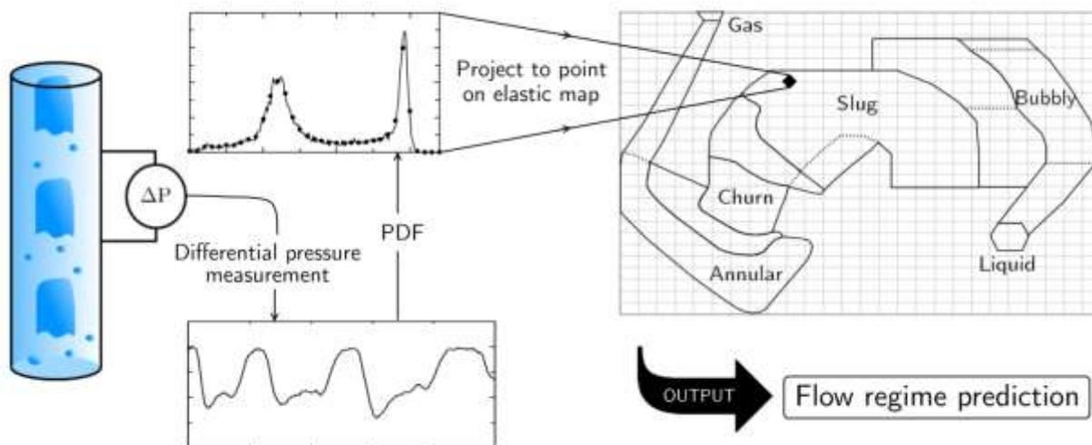
Figure 3: Illustration of newly proposed flow regime prediction method.
