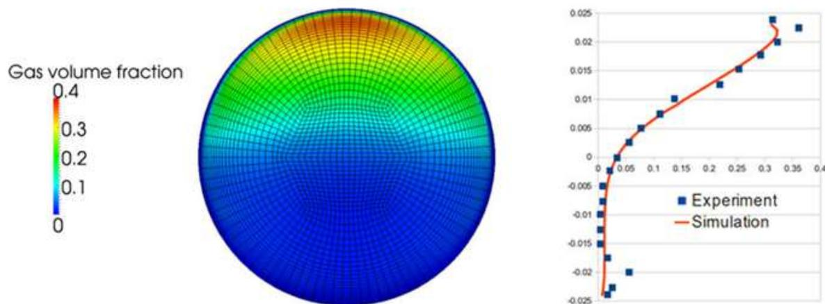
Figure 4: Void fraction map at the pipe outlet (left) and comparison with experiment (right).
